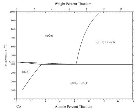
Fig. 1 Co-Ti phase diagram
